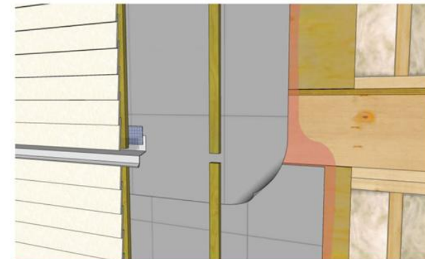
Figure 2-37. Self-adhered sheathing membrane with adhesive primer.
